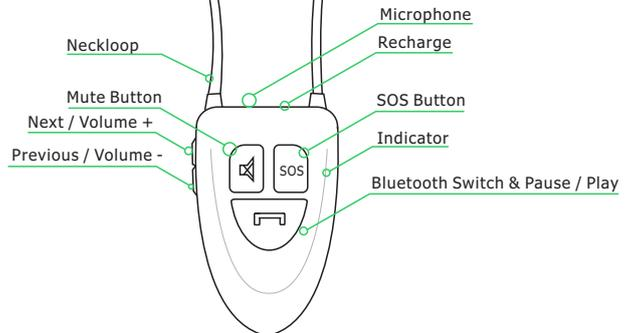
Bluetooth neckloop is build as F class low consumption audio amplifier. Power of amplifier is 3.5watt. It can support all kinds of wireless earpieces and provides very loud audio sounds.
